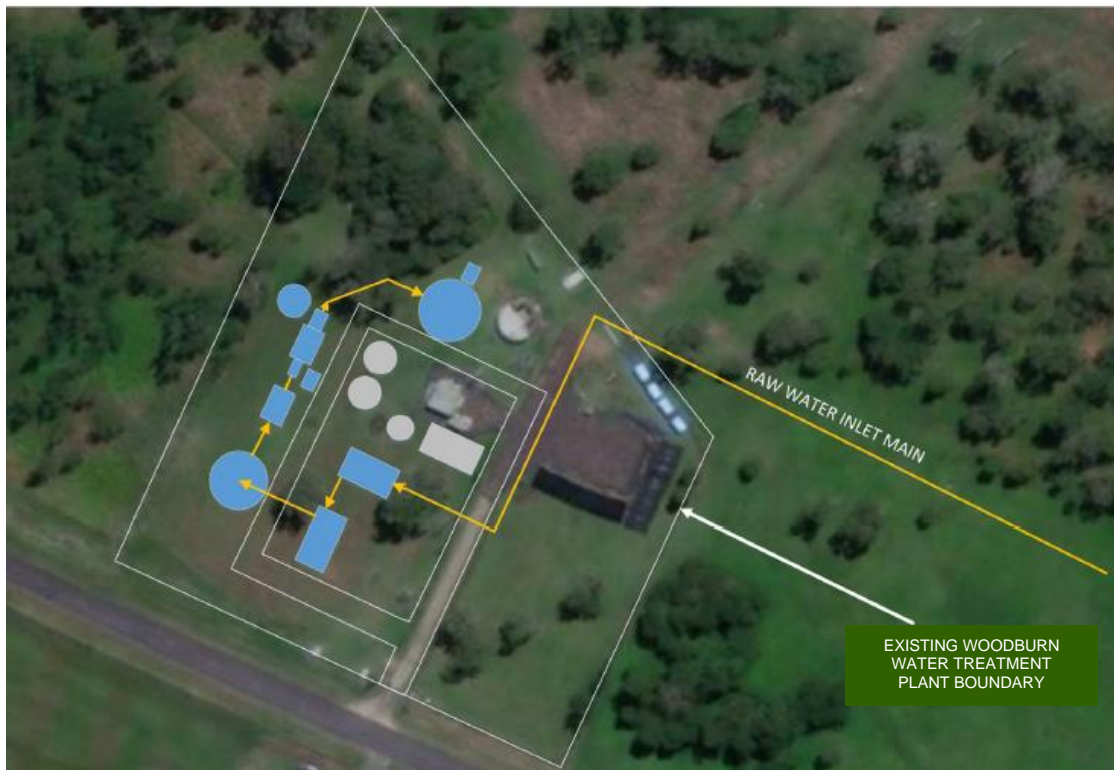
Figure 14: Woodburn groundwater WTP inlet and layout
